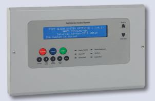
The XL-RDU, LCD remote display repeater panels have the same, easy to use, controls and indications as the main control panels with the addition of a 4 line x 40 character, backlit LCD display.
