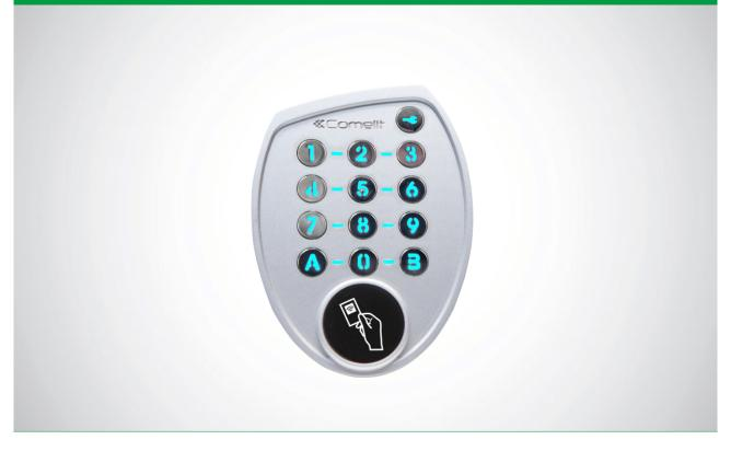
Anti-vandal electronic key code in zamak, 100 codes of 3 to 6 characters, backlit buttons. With integrated RFID reader, Mifare technology. 500 proximity keys can be programmed and configured once learned. Configurable relays in monostable mode from 1 to 99 seconds or in bistable mode. Exit button, clock and alarm management. Opening with code, badge or code and badge. Option of external relay connected to RS485 serial line. Temperature from -25°C to +55°C, IP54. Dimensions 122 x 90 x 19 mm.
