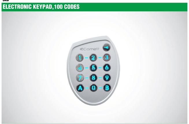
Anti-vandal electronic keypad in zamak, 100 codes of 3 to 6 characters, backlit buttons. Configurable relays in monostable mode from 1 to 99 seconds or in bistable mode. Exit button, clock and alarm management. Optional external relay connected to RS485 serial line. Operating Temperature from  $-25^{\circ}$ C to  $+55^{\circ}$ C, IP54. Dimensions  $104 \times 80 \times 19$  mm.
