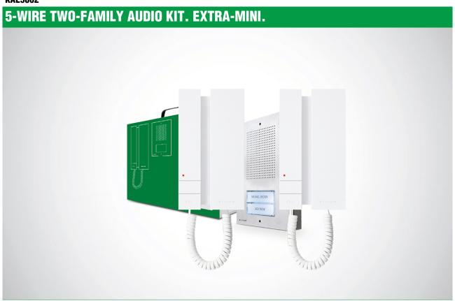
The kit includes: two Mini series door-entry phones art. 2702W, one transformer art. 1200, one Extra series external unit with 2 call buttons art. ET5002. The kit can be expanded with another door-entry phone for each user. The external unit can be surface-mounted or flush-mounted using the relevant accessories supplied with the kit.
