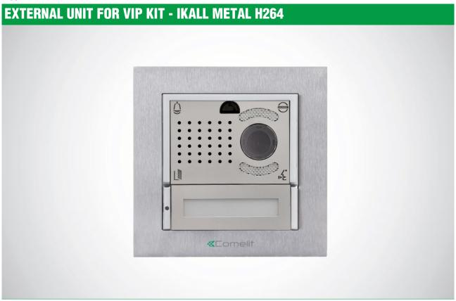
Single-family video door entry external unit for ViP system with Ikall Metal entrance panel. The kit comprises: 1 flush-mounted box Art. 3110/1, 1 silver coloured frame Art. 3311/1S, 1 module with 1 button art. 33411M and 1 colour audio/video unit Art. 4682HKC. The external unit is coded with ViP address 100 and the button on module Art. 33411M sends the call to ViP address 1. Compatible with H264 video format
