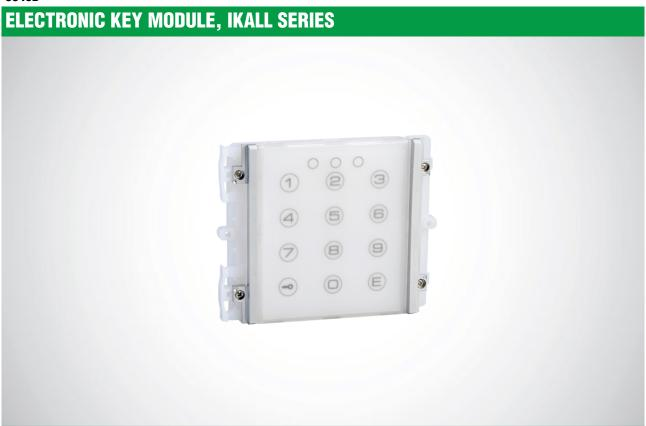
Digital electronic key module with LED keypad backlighting. Blue, white and off lighting options. When a number with between 1 and 8 digits is entered on the keypad, two relays (10A) are activated, allowing the operation of electric door locks or other devices. Dimensions 112x89.5x40 mm.
