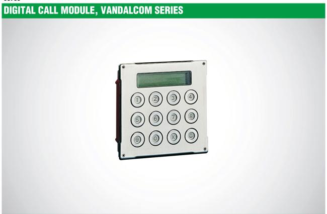
Module made using double 2.5 mm 316 stainless steel plate, complete with keypad featuring 12 backlit buttons and 16-digit alphanumeric display showing call codes and user interaction messages (busy, etc.). Also functions as an electronic key code with 1000 possible different 6-digit command codes. Dimensions: 106x106x56 mm. Compatible only with the art. 4680, 4680C, 4681, 4682HC, 1621, 1621VC, 1622, 1622VC, 1682 and 1682HVC combined with the fronts art. 3262S/x and 3268S/x.
