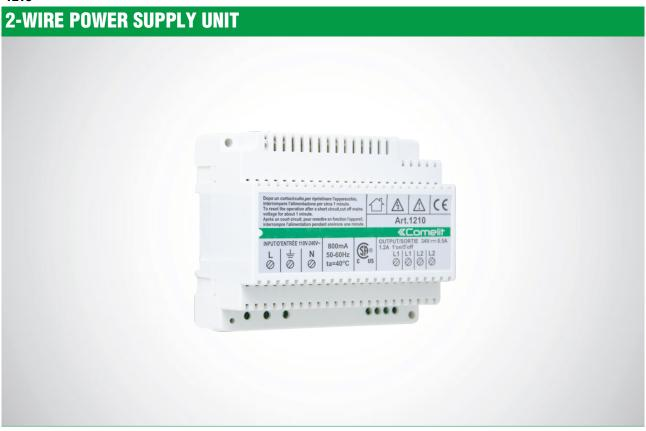
2-wire power supply unit required to power the external unit (terminals L1 - L1) and the support column (terminals L2 - L2). Equipped with 1 terminal for line termination art 1216. Input voltage 110-240Vac. Compatible with audio/video unit art. 4681 and 1621VC and audio unit art. 1621. Dimensions: 106x89x62mm (6 DIN modules).
