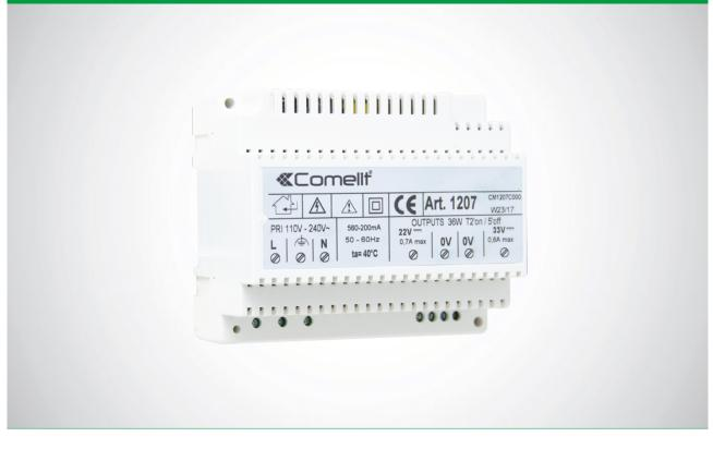
Power supply unit with overload and short circuit protection devices. It has two separate continuous outputs: 33vDC for external unit and 20V DC for the monitor power supply. Input voltage 120-230 VAC. Dimensions: 105x85x85 mm (6 DIN modules).
