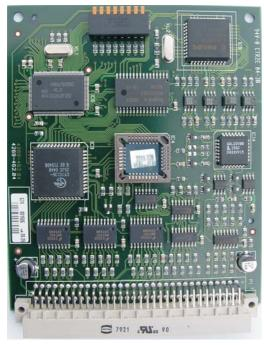
This copper network card is used to allow messages of status and control data to pass between control panels and network (or terminal) nodes in a networked fire system. The card must be plugged into the backplane of each panel and node in a dedicated slot. When it is plugged into the slot P8 on the backplane the external cables must be connected to terminal block P10, which is also located on the backplane.
