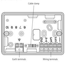
The TRTM7 is supplied with a standard back box, which can be used if there is no existing back box already installed. The new back box may be screwed to the wall using the fittings provided.
