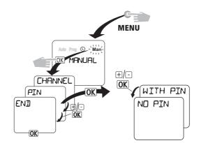
If a PIN code has been activated, the timer can no longer be activated without a valid PIN code after a RESET.
