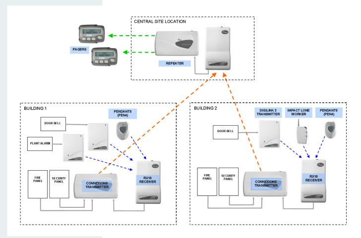
An integrated system utilising a repeater in a central location to ensure full site coverage to the pagers. The system monitors the fire and intruder alarms as well as pendant alarms, lone workers and other devices
