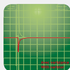
ELECTRONIC PROTECTION TO ELIMINATE BACK EMF (VARISTOR SUPPLIED)
