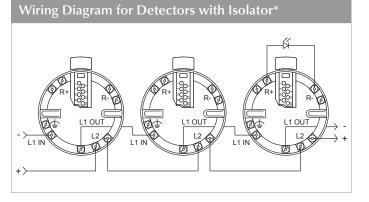
\*Note: Detectors without isolators will work with the above connections, however if there are no isolators in the system or it is a retrofit application, the arrangement below is recommended.
