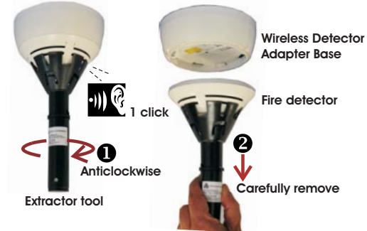
Removal of Wireless Detector Adapter Base with Detector
