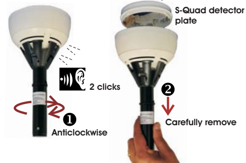
Removal of Wireless Detector Adapter Base with Detector
