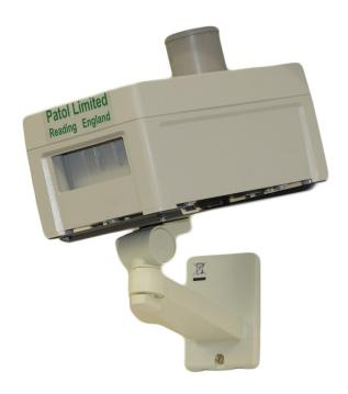
The 5730 High Temperature Transit Flame Sensor monitors high temperature materials (up to 240° on highest sensitivity), being transported on conveyor systems at speeds of between 0.5 and 6m/s, and triggers as the material reaches the ember or flame condition.
