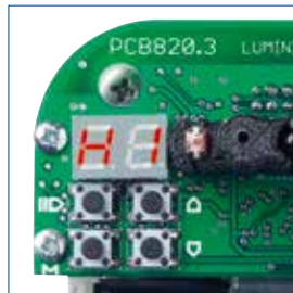
New easy access programme feature with LED display makes set up and testing very simple.
