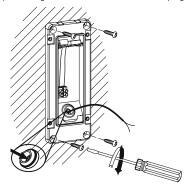
Terminate the cable into the terminal block (See section 5. Connection Diagram) ensuring correct polarity is observed and that all bare conductors are sleeved.
