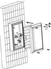
Note: 4 Allen bolts are also supplied which can be used instead of the four Pozi screws if required. If used a 3mm Allen key is required. You are also able to change the bezel at this stage using one of the alternatives listed at the beginning of these instructions — Sold separately.
