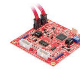
996520PCB&K Integriti UniBus 2 Port RS-232/RS-485 UART PCB & Accessories (Includes 270mm UniBus patch cable)
