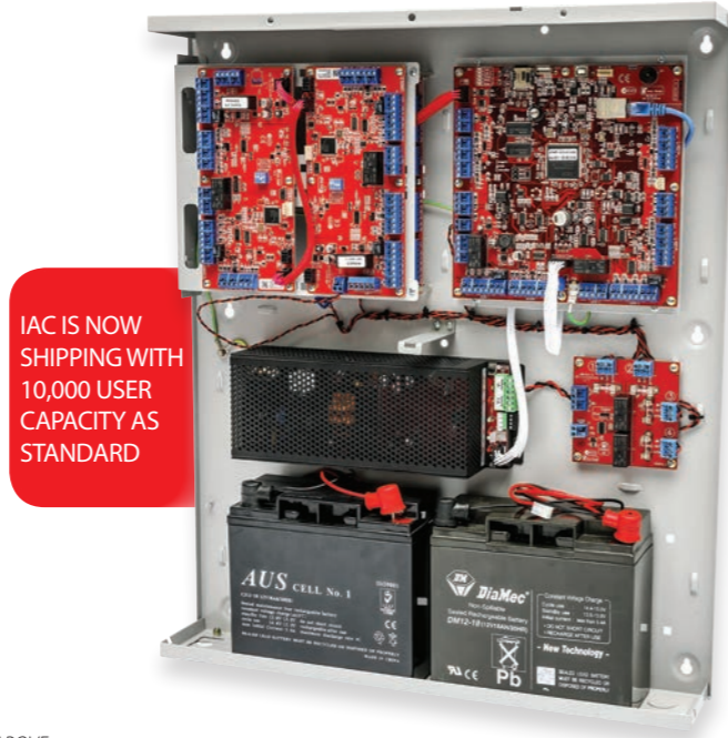
ABOVE: IAC shown in 8 Door / 10 Reader configuration. (IAC with UniBus 2 Door / 2 Reader expansion devices connected). Housed in the WideBody enclosure with hinge plate, 8Amp PSU, Fire Door override relay card and 2x 17Ah batteries
