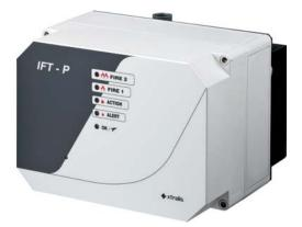
The ICAM IFT-P detector is an air-sampling system with an alarm sensitivity range from 0.001% to 20% obscuration/m (0.0003% to 6.10% obscuration/ft). This detector is classified as a Very Early Warning Smoke Detector that can reliably detect fire at an early stage, and low to high concentrations of smoke over an area of up to 2000 m<sup>2</sup> (21 500 ft<sup>2</sup>).
