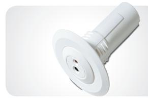
The GS903N detects in a full 360° coverage pattern with a 7.5 m range from detector to glass. By listening at more than 30 frequency points, the GS903N can tell the difference between common false alarm sources and the noise of breaking glass.
