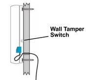
Figure 3 Mount the Transmitter to the Wall
