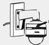
D: Fastening screw of dome camera
