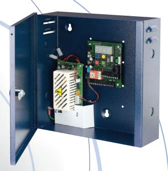
The Solo 2 from Controlsoft is a standalone Access Control Unit, providing cost effective access control for two door applications using Wiegand readers.
