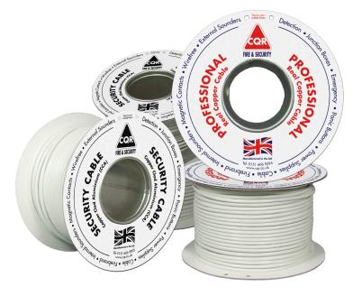
This UK manufactured cable has cores of 7 strands of 0.182mm annealed tinned copper wire and is sheathed in Type 1 PVC. Suitable for any installation where signal integrity is paramount.
