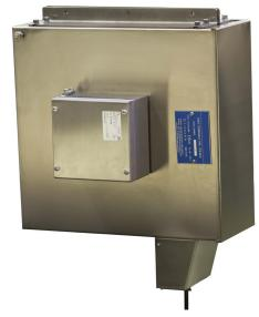
A rim seal fire detection system using Linear Heat Detection Cable (LHDC) can be installed at the edge of the rim seal of a floating roof tank. An automatic cable reeler provides the electrical connection between LHDC and control panel and accommodates the rise and fall of the floating roof.
