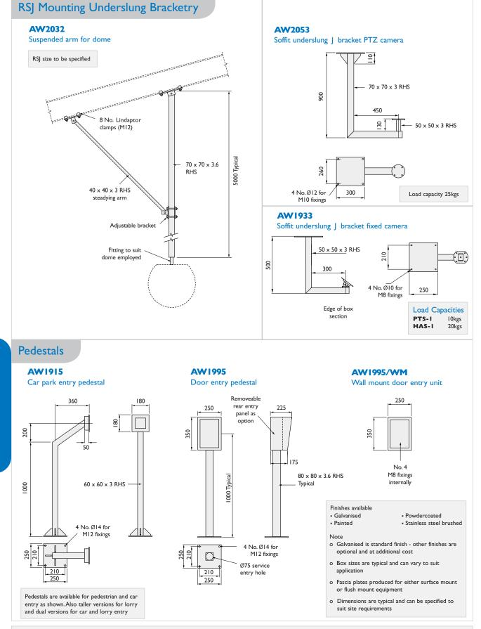
All brackets for camera mounting have a Ø127 mounting plate with 8 no Ø8.5 equi - spaced on 101.6 PCD
