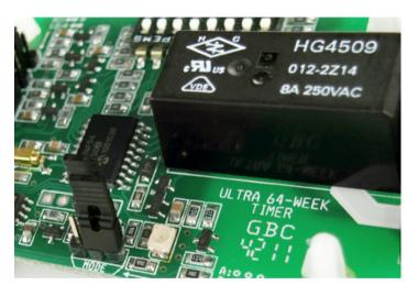
however if the door is open after the 3 minutes the relay will activate - if auto link is fitted relay drops out after 20 seconds and is then "waiting for next trigger"
