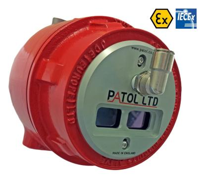
The 5710 High Temperature Transit Flame Sensor monitors high temperature materials (up to 240° on highest sensitivity), being transported on conveyor systems at speeds of between 0.5 and 6m/s, and triggers as the material reaches the ember or flame condition.
