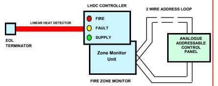
Notes: Configurations for Fig 2 & 3, is dependant on the voltage and current specifications of the LDM-519-LP being compatible with the monitoring technique and electrical characteristics of the Control Panel / Zone Monitor.
