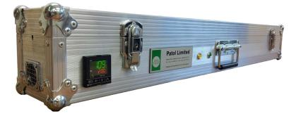
Commissioning and routine maintenance testing of the Patol Analogue Linear Heat Detection Cable systems can be conducted at site by the use of a calibrated 1 metre test oven.
