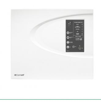
Eracle 2 zones is a conventional fire alarm panel certificated by EN54-2 and 4. Up to 32 detectors and manual call points can be connected to each fire zone. The panel is provided with robust plastic cabinet and with LED display. The panel shows fire and faults alarm for each detection zone plus generale information such as alarm, fault, sounder disable, zones disable, test, power. Commands available are test, sounder silence, reset, walk test. Access protected by key.
